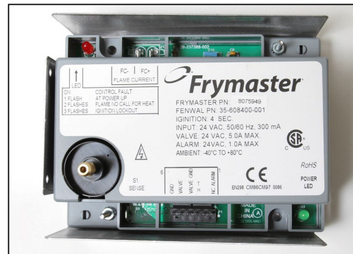
Figure 1 Fenwal 8075949 Ignition Module
